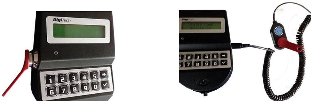
If the DigiTech was previously programmed to have a reset security code, the LCD display of the keypad will show the message **RESET CODE**, then you have to enter the reset code. If you enter a wrong reset code, a message will inform you that the reset code is wrong and the operation will be aborted.
