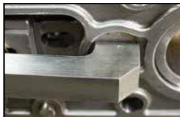
Milled oblong circle on the Inside Back Plate Fixture seats the clamp portion
