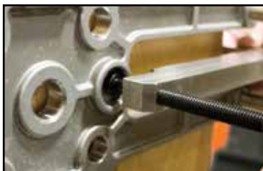
Milled circle on the Front Plate Fixture seats the clamp's screw.
