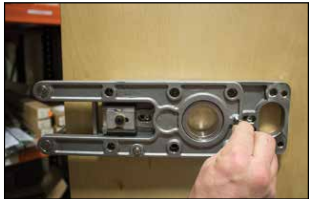
Step 8 - Seat the Back Plate Fixture over the locator pin and tighten the wing nut.
